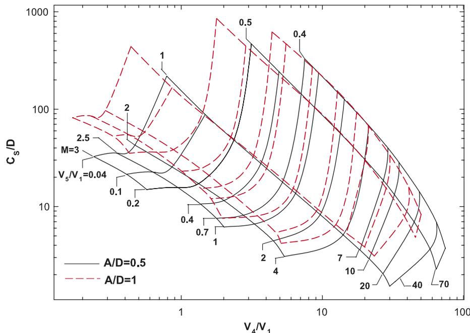
Fig. 10. The spherical aberration coefficients,  $C_s/D$ , as a function of  $V_4/V_1$  in terms of the magnification  $M$  and  $V_5/V_1$  for  $A/D = 0.5$  ( $L/D = 2.5$ ) and 1 ( $L/D = 3$ ) (see Fig. 14 of Ref. [31] for voltage ratios).
