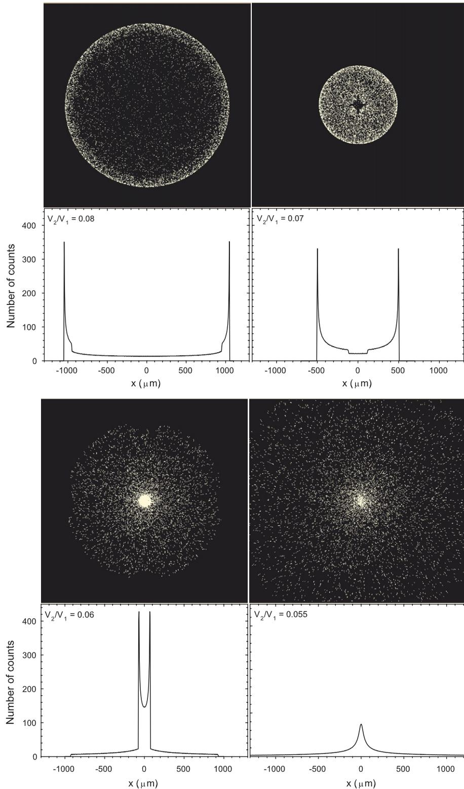
Fig. 4. Distribution of electrons at a fixed image distance for a two-element lens with  $P/D = Q/D = 2$  for four different voltage ratios,  $V_2/V_1 = 0.08$ , 0.07, 0.06 and 0.055 (see text). The optimal focus point corresponds to the case for  $V_2/V_1 = 0.06$ .
