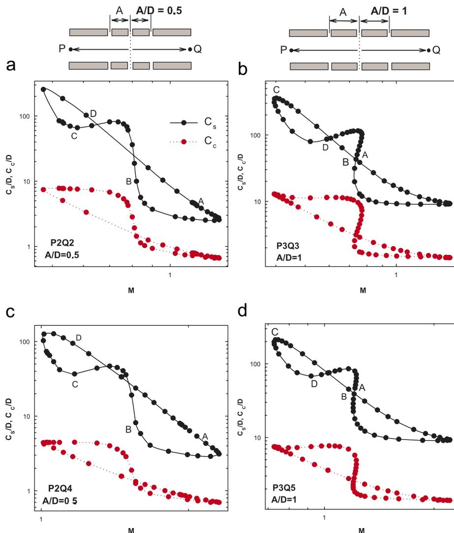
Fig. 7. Values of the spherical and chromatic aberration coefficient  $C_s/D$  and  $C_c/D$  for four-element lenses with (a)–(c)  $A/D = 0.5$  and (b)–(d) 1 as a function of the magnification for different values of  $P$  and  $Q$  (see Fig. 8 of Ref. [31] for voltage ratios).
