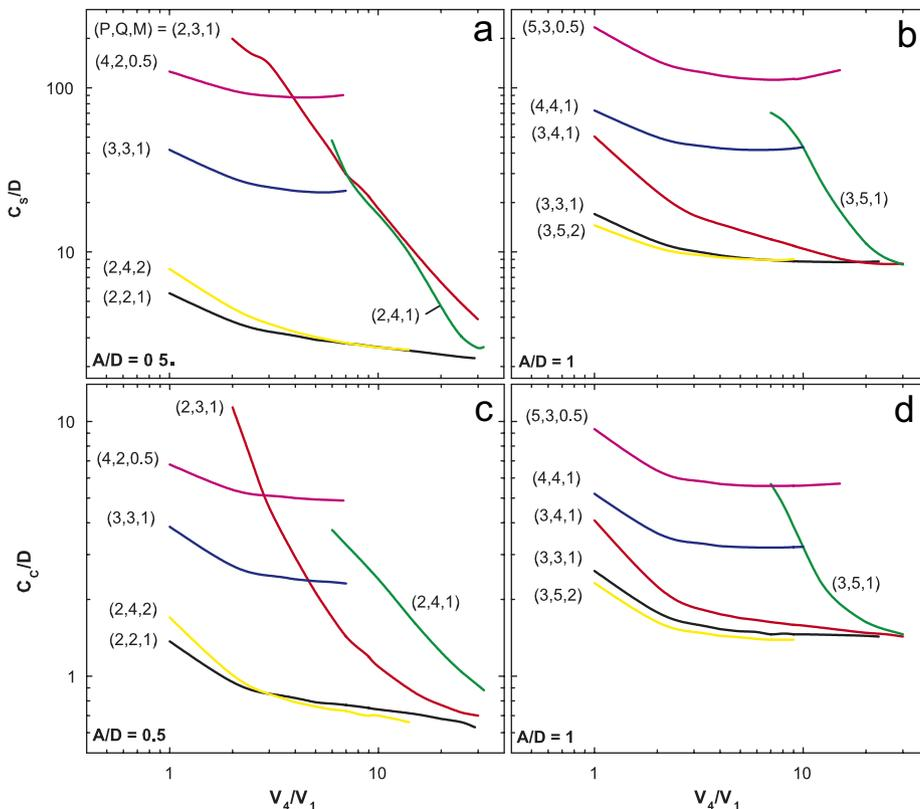
Fig. 8. Values of the (a)–(b) spherical and (c)–(d) chromatic aberration coefficient  $C_s/D$  and  $C_c/D$  for four-element lenses with  $A/D = 0.5$  and 1 as a function of  $V_4/V_1$  for six combinations of  $(P, Q, M)$  (see Fig. 9 of Ref. [31] for voltage ratios).
