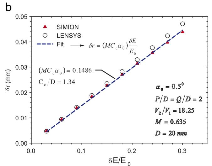
Fig. 3. Calculations of the aberration coefficients  $C_s$  and  $C_c$  of a two-element lens for  $P/D = Q/D = 2$  and  $V_2/V_1 = 18.25$  using the ray-tracing simulation programs SIMION and LENSYS. The aberration discs  $\Delta r$  and  $\delta r$  are recorded as a function of  $\alpha_0$  and  $\delta E/E_0$ , respectively.
