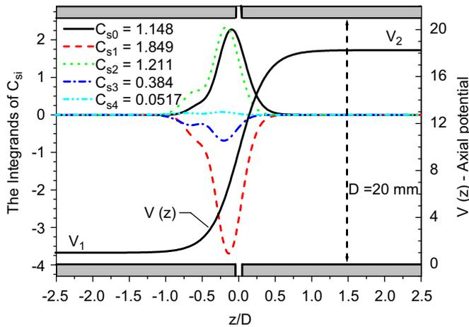
Fig. 2. The integrands for each spherical aberration coefficients  $C_{si}$  and axial potential  $V(z)$  for a two-element lens with an acceleration voltage 1 : 18.25 for  $P/D = Q/D = 2$ . The individual curves can readily be associated with particular coefficients and for this lens they are, from the top,  $C_{s0}$ ,  $C_{s2}$ ,  $C_{s4}$ ,  $C_{s3}$ ,  $C_{s1}$ .
