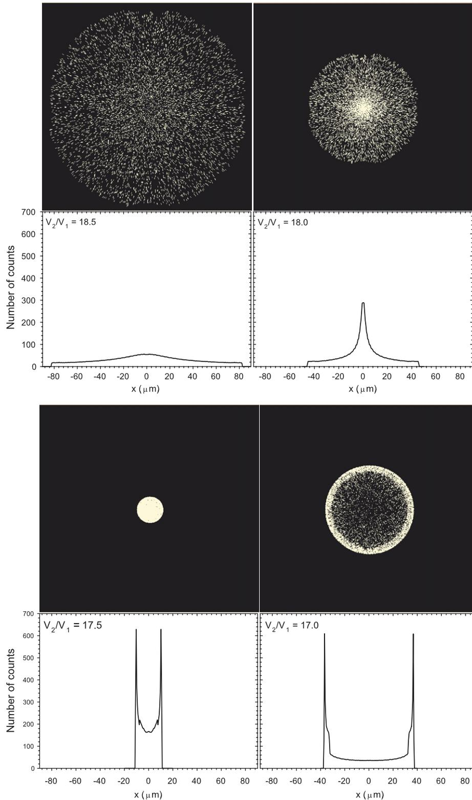
Fig. 5. Distribution of electrons at a fixed image distance for a two-element lens with  $P/D = Q/D = 2$  for four different voltage ratios,  $V_2/V_1 = 18.5$ , 18.0, 17.5 and 17.0 (see text). The optimal focus point corresponds to the case for  $V_2/V_1 = 17.5$ .
